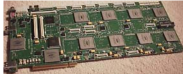
Figure 3. Top view of the 3D-Flow™ DAQ IBM PC photon detection board.
